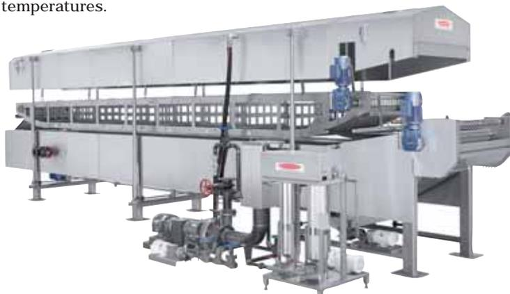
**CHOOSE CORRECTLY:** Pick a fryer based on your-energy, heater, cleaning and oil-filtration requirements.
