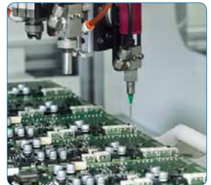
Conformal coated circuit boards resist damage from internal condensation.
