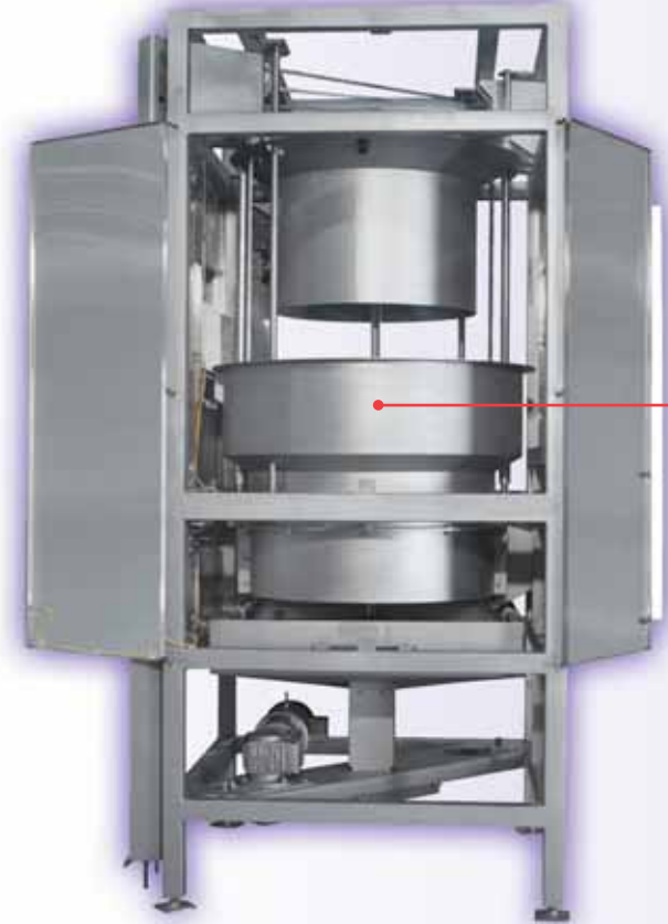
Doors on both sides provide easy access to abrasive drums, disc and drive system. Two drive bearings are lubricated via external fittings.
