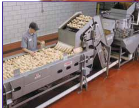
Two-stage batch peeling improves peeling control for higher yield and better product quality.
