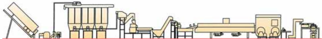
Continuous System up to 6,500 lbs/hr regular, low-fat and fat-free potato chips
