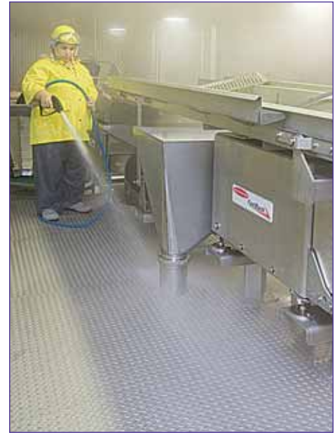
Sloped deck provides superior sanitation.
