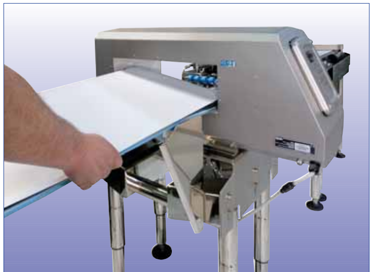
Remove conveyors without using tools for easy cleaning and service.
