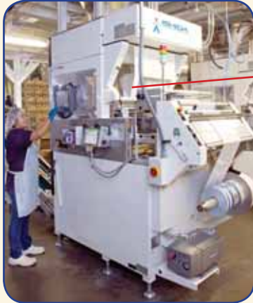
Ishida AFT kit includes tracking photo eyes, digital readout, control software, mounting hardware, and wiring.
