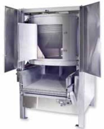
◀ *As chips leave the batch fryer, they are gently conveyed to the Automatic Heated Centrifuge (shown at left).*
