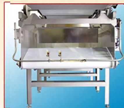
Internal let-down chute option & sloped discharge belt minimize product breakage.
