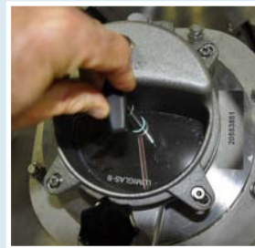
Illuminated view ports permit observation of product during operation.
