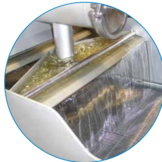
Curtains of filtered oil enrobe products, transferring heat quickly and uniformly.
