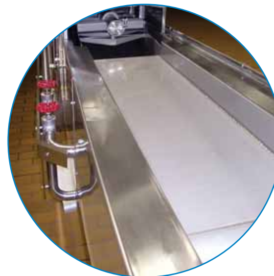
Drop-in infeed flume extensions allow delicate batter coatings and noodles to set before final frying.
