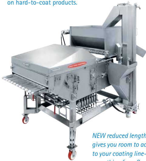
Triple-Flip conveyors assure uniform coverage on hard-to-coat products.
