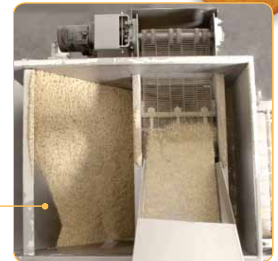
Sifter conveyor removes lumps from non free-flowing breading hopper.
