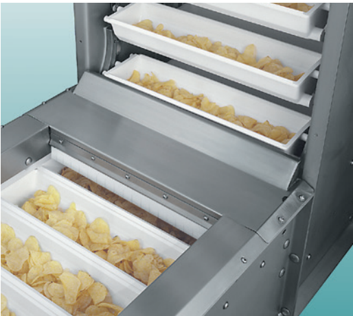
Overlapping buckets prevent product loss during loading.
