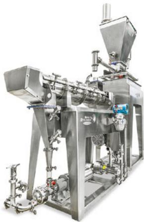
Slurry On Demand Continuous Mixer, an alternative to traditional mix/use tank option. Reduces slurry waste at the end of production run.
