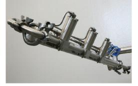
Slurry spray manifold with hard-piped air lines between spray stations
