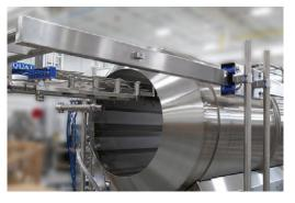
Optional manifold trolley pull out assembly
