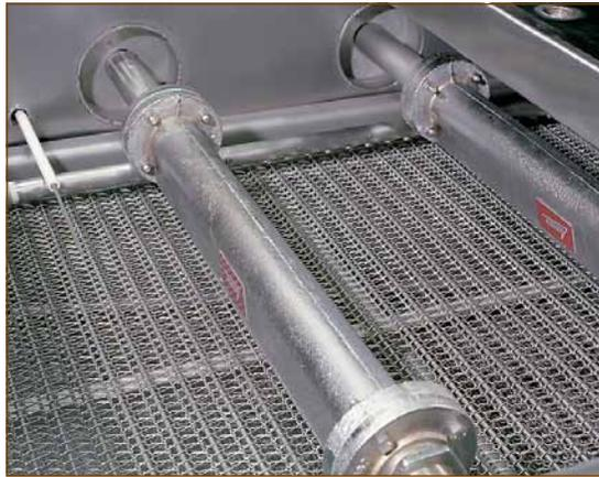
Water sprays remove debris from the conveyor belt to simplify cleaning.
