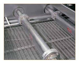
Water sprays remove debris from the conveyor belt to simplify cleaning.
