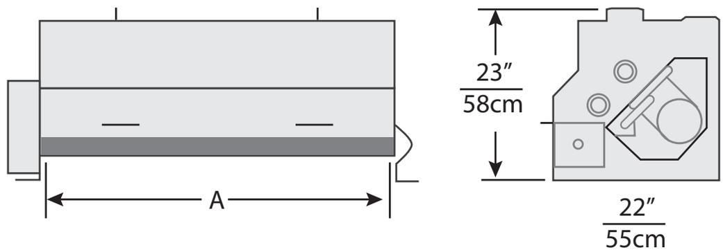
Models available in salting widths (A) from 24" to 78" (61cm to 198 cm)
