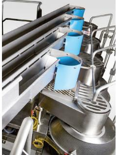
Potatoes are metered at a consistent rate for efficient feed and line operation.
