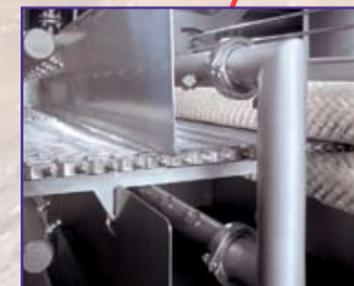
*Rotary brushes, water sprays, and air blowoffs continually clean and dry the conveyor belt.*
