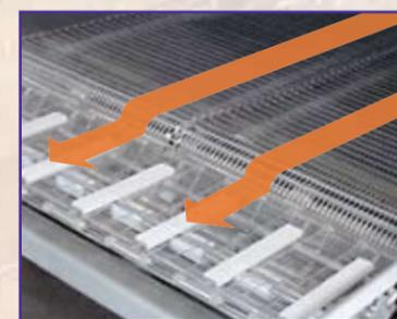
*Discharge/infeed transfer conveyors prevent product damage during transfer. Lecithin applicator is available on infeed belt to reduce product sticking.*
