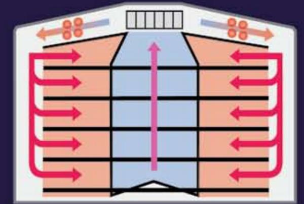
*Centered inside the top of the cylindrical enclosure, one fan circulates the cooking atmosphere in a 360° pattern evenly across all conveyor tiers.*
