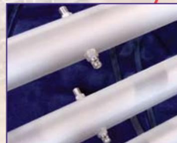
*Clean-in-place sprays are built into the conveyor support framework to thoroughly clean both sides of the belt.*
