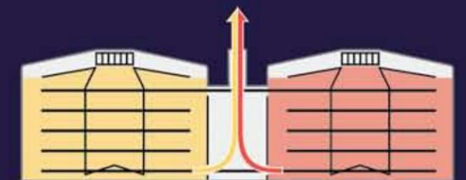
*On two-zone models, venting exhaust through a central stack prevents the cooking atmosphere from migrating between zones. Steam only, dry heat, or any combination can be controlled independently in each zone without affecting the other zone.*
