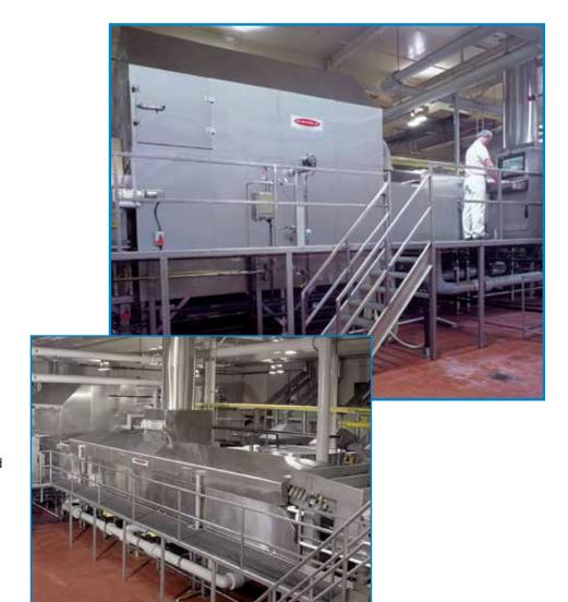
The Low-Fat Stripper mounts to the discharge of the fryer enabling your existing line to produce reduced-fat, fat-free and regular fried products.
