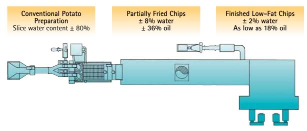
Heat and Control supplies the complete system plus worldwide parts and technical support.
