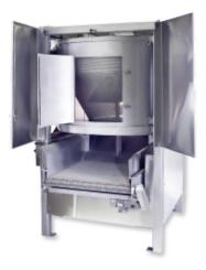
As chips leave the batch fryer, they are gently conveyed to the Automatic Centrifuge (shown at left).
