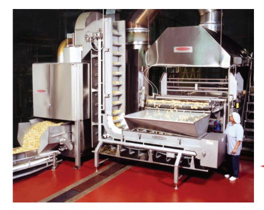
Reduce the oil content of batch fried potato chips to 22% or less, depending on the potatoes' specific gravity.
