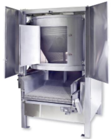
◀ *As chips leave the batch fryer, they are gently conveyed to the Automatic Centrifuge (shown at left).*
