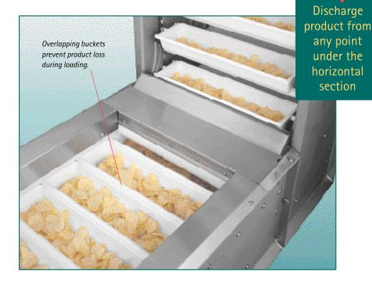
Tip-To-Clean™ option aligns buckets in dump position for easy floor-level cleaning.
