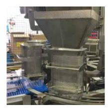
**Tray loading into Rotary hopper**
