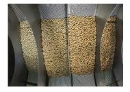
First-In-First-Out performance with stepspiraled and flighted drum.
