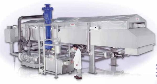
4,200 finished lb/hr Multi-Zone Fryer with KleenSweep® centrifugal oil filter.
