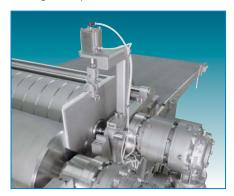
Red tape switches stop the sheeter immediately and are easily accessible across the full width of the front and rear rolls.
