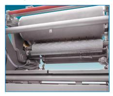
Pneumatically controlled containment saddles prevent masa leaks. Pneumatic controls also adjust stripping wire, cutter, brush, and discharge conveyor.
