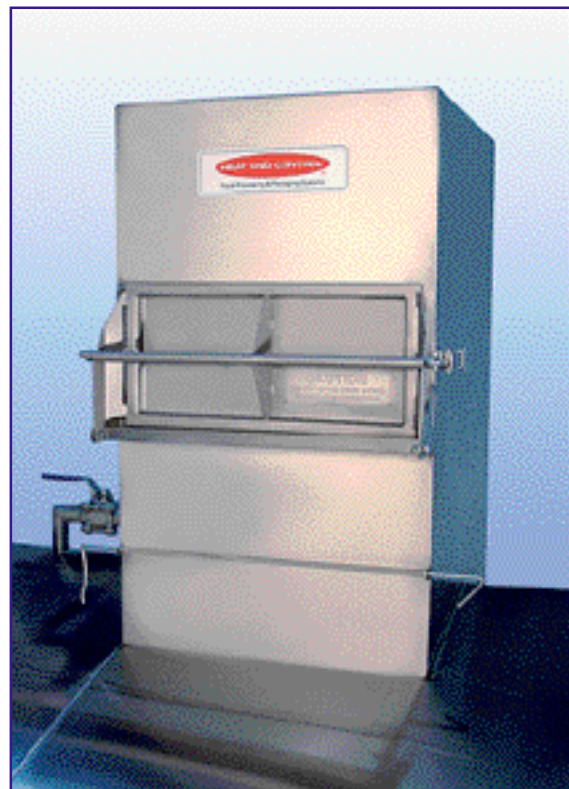
Hinged door allows easy pad replacement.
