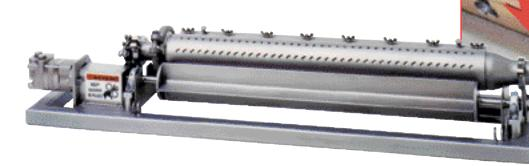
Nugget sizes are easily changed with a rotating sleeve. Choose electric or hydraulic drives.
