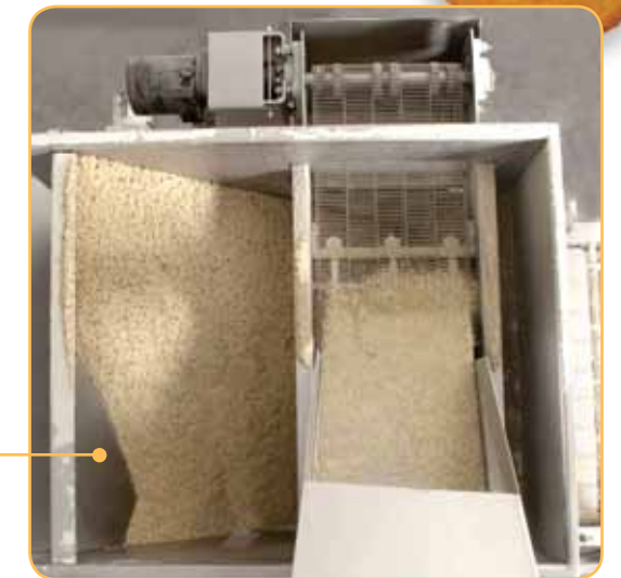
Sifter conveyor removes lumps from non free-flowing breeding hopper.
