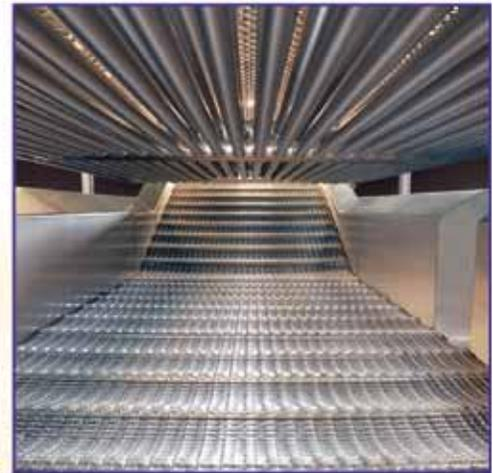
*Heat transfer tubes and hood can be lifted clear of the fines removal conveyor to simplify cleaning.*
