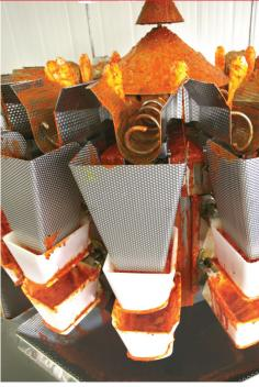
Additionally, sturdy, non-stick plastic hoppers fitted with scraper doors prevent product build-up and keep the product moving. The company's marinated chicken line has increased to 35 weighments per minute, a rate similar to a free-flowing product.
