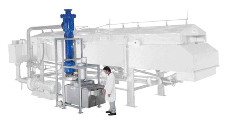
Continuously remove particles as small as 250 microns from frying oil for snacks, french fries & batter-breaded foods.
