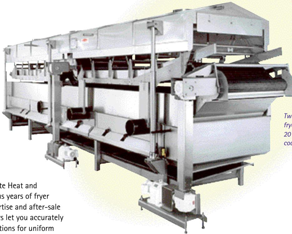
*Two-stage multi-zone fryer produces up to 20 tons/hour of batter coated or regular fries.*
