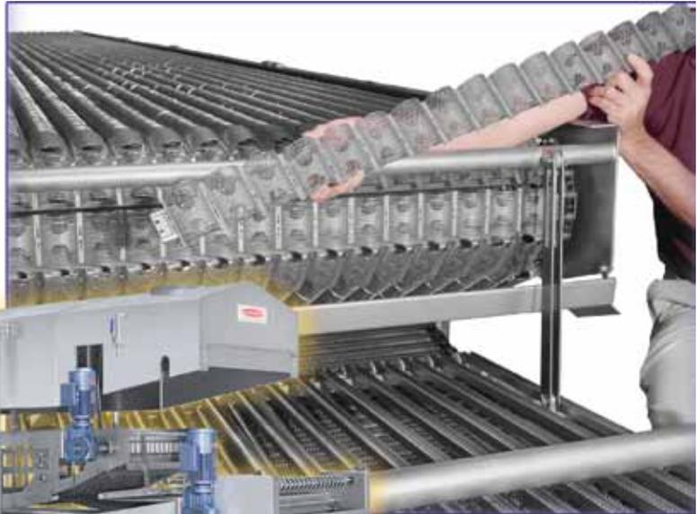
*Chip molds are easily removed. Shown with an optional Canister Filter, fryers are available with a variety of oil filters to suit your product.*
