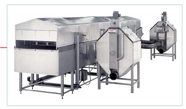
Drum Pre-Filters are easily installed on existing single and multi-stage fryers.
