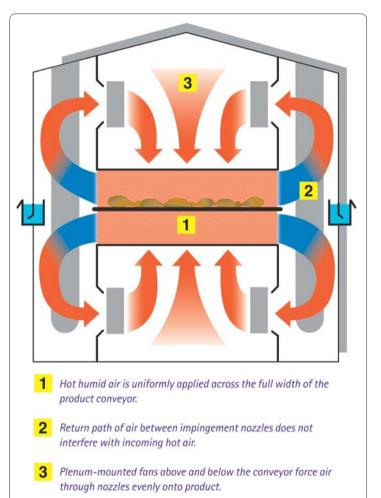
Typical air flow diagram inside the Airforce Impingement Oven.
