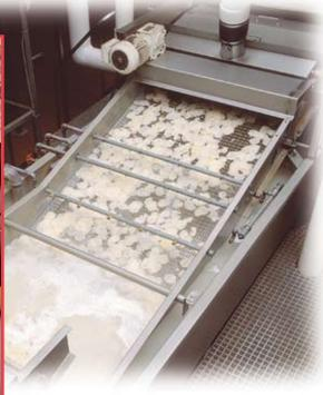
Standard models fit conveyor belts up to 60" wide. Custom designs, like this dual air knife system (left) are also available.
