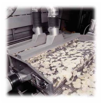
For maximum removal of surface water and particles, our AirSweep dewatering system conbines the Air Knife with a vacuum plemum.
