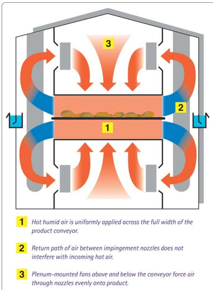
*Typical air flow diagram inside the Airforce Impingement Oven.*
