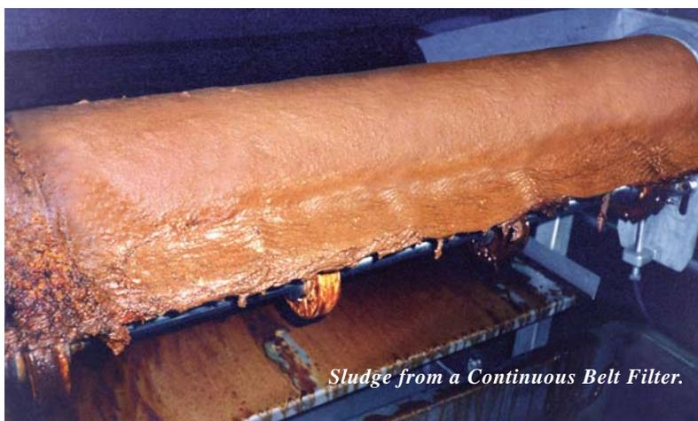
*Sludge from a Continuous Belt Filter.*
