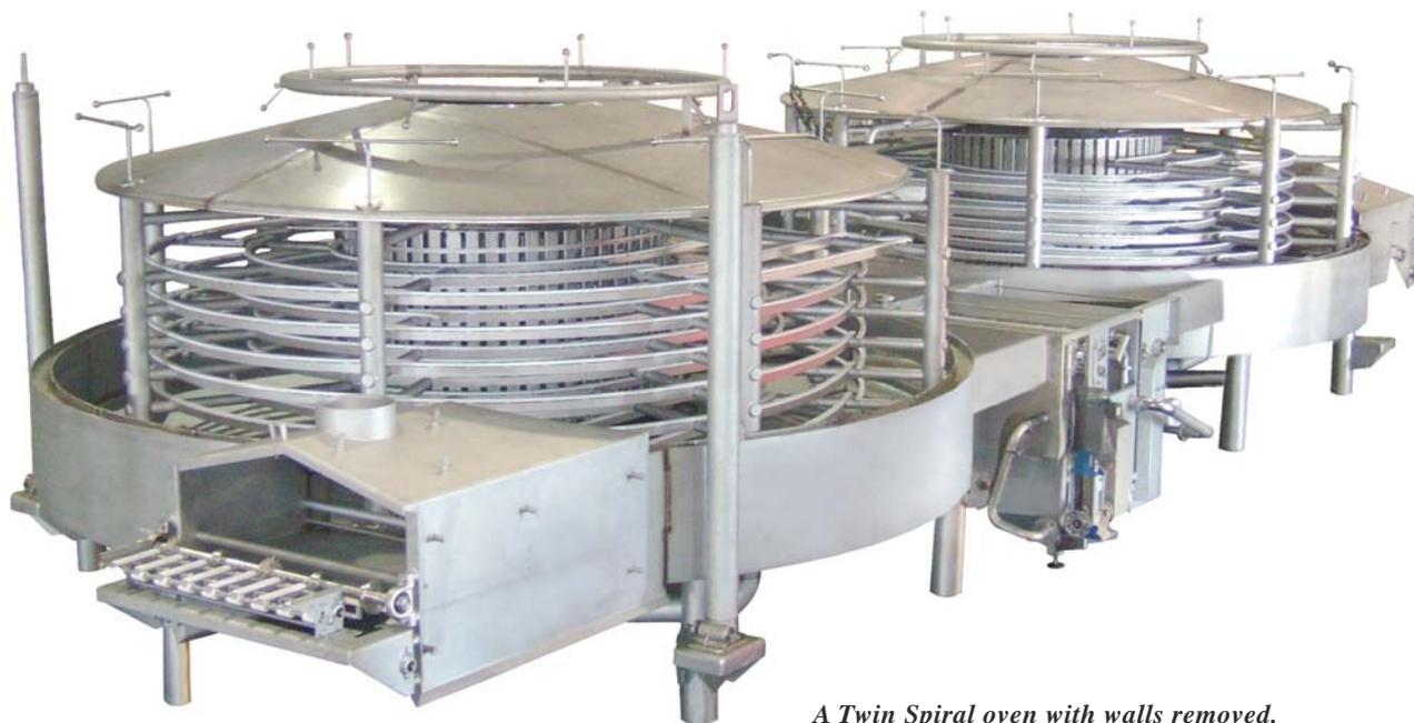
*A Twin Spiral oven with walls removed.*
