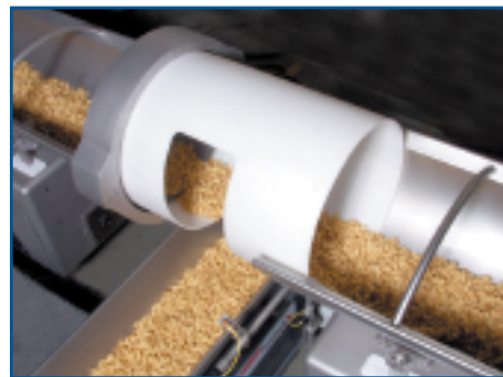
As product flows in the main distribution line, Revolution rotates to divert a portion to individual weigher/bagger stations without cutting the supply to other units.
