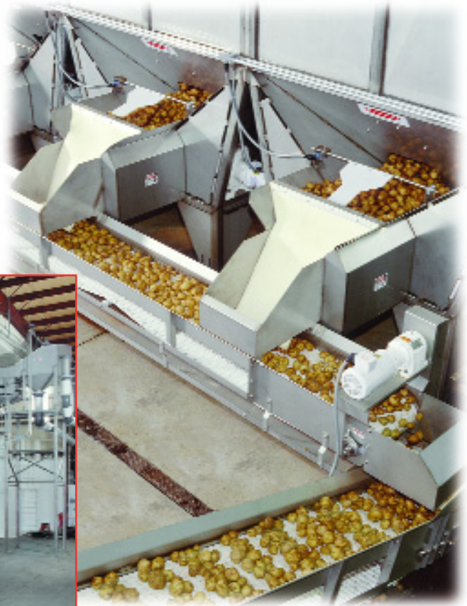
Bins are available in painted or stainless steel construction with a belt or auger discharge.
