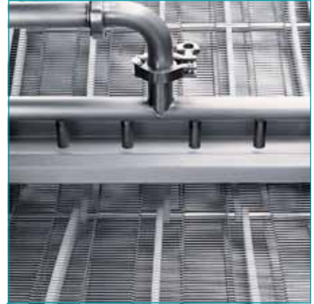
Two or four curtain batterfall option assures uniform coverage of formed products, vegetables and bone-in poultry.
