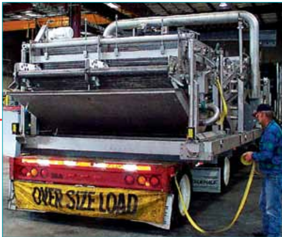
With a 96" wide belt, this 40,000 pounds/hour coating system is designed for 24-hour-a-day operation.
