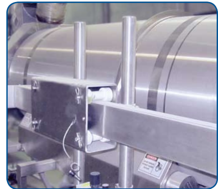
Optional Easy Pull™ spray bar mount allows safer "tools-free" installation and removal of the spray bar and/or Uni-Spense.
