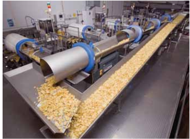
Uphill horizontal motion conveying reduces product damage in return loops.
