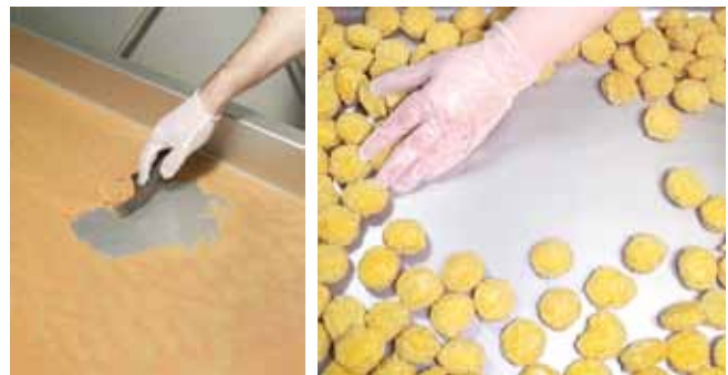
Coatings build up on a vibratory conveyor pan (left), but not on horizontal motion conveyors (right).
