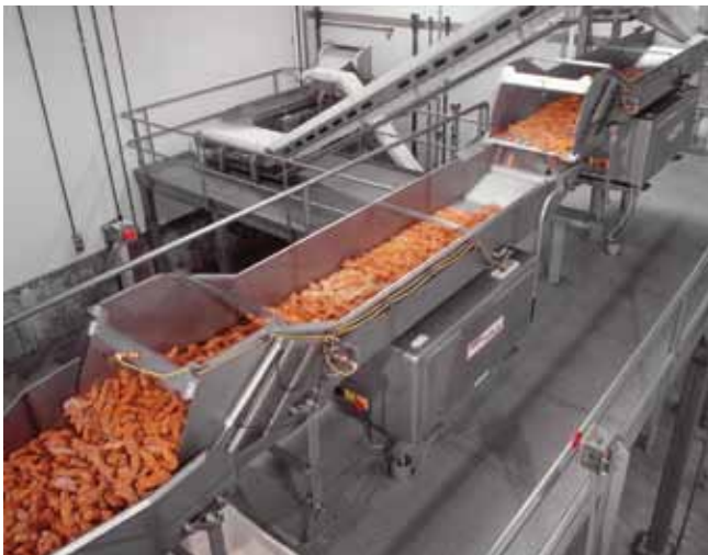
Horizontal motion allows gentle short term product accumulation.
